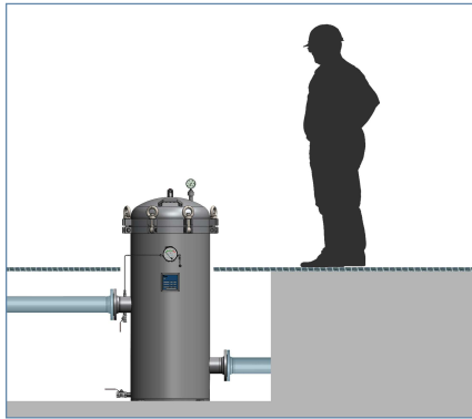
shaft / overflow basin installation
